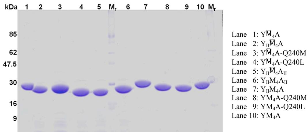
**Figure S6:** Single-step IMAC purification of YM/ $\overline{M}_4$ A N- and C-cap variants. The expected size is approximately 27 kDa. Proteins were analyzed by SDS-PAGE (15%). The size marker is indicated in kDa.
